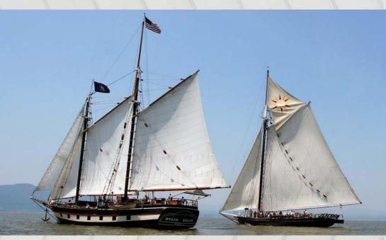
(RIGHT) Built of traditional plank-on-frame wooden construction, the sloop Clearwater is 75 feet in length on deck, 25 feet in beam and can hold up to 70 tons of cargo. The sloop rig consists of a single mast and fidded topmast which together rise to a height of 108 feet, a 65-foot long main boom and a 28-feet long bowsprit.
